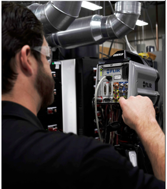
Taimen Taylor, Sales Engineer at Teledyne FLIR, sets up a high-speed thermal camera to monitor battery testing.
