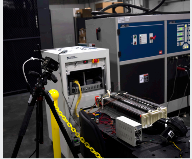
FLIR A70 thermal camera monitoring testing on a battery pack.
