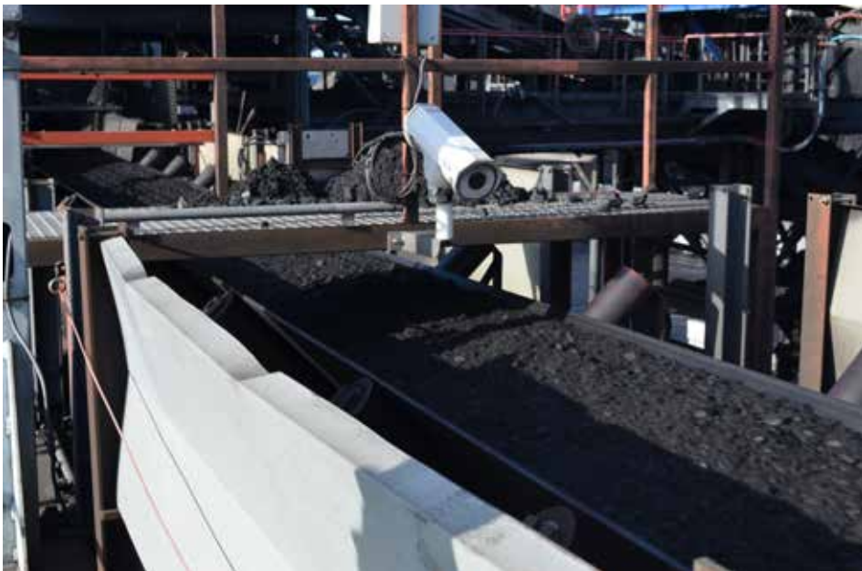
When the coals are on the conveyor belt, thermal imaging cameras allow us to see temperatures of the entire coal mass, not just of the coal surface.
