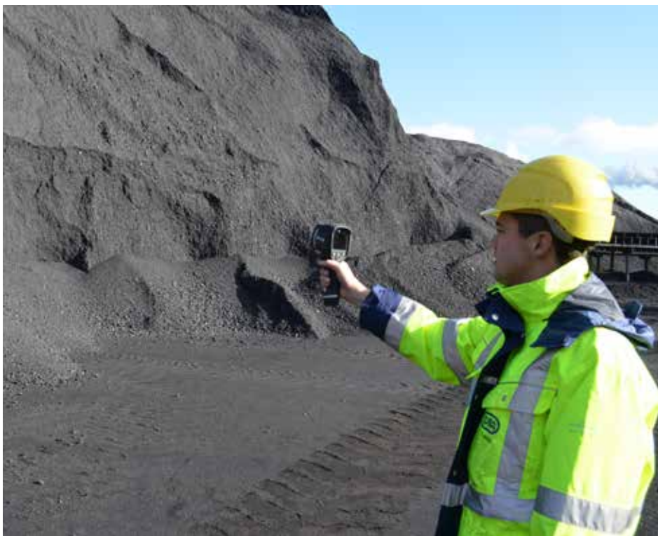
OBA combines the use of a temperature probe – the traditional way of measuring temperatures – and a FLIR E6 handheld thermal imaging camera.
