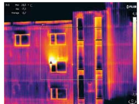
*When inspecting higher multi-story buildings, the drone can even take thermographic images of the facade at the 10th floor and with the highest level of discretion because window glass is nontransparent for the thermal imaging camera.*
