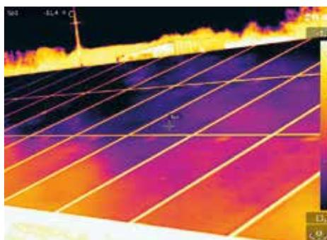
*Due to the high thermal resolution of the FLIR T640bx thermal imaging camera with permanent autofocus, MSX function and a full range of features, the drone detects problem areas in photovoltaic modules from the air.*
