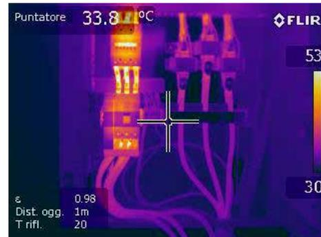
Thermal imaging cameras can be used to inspect all components of a photovoltaic installation, including inverters, fuses, cables and connections.
