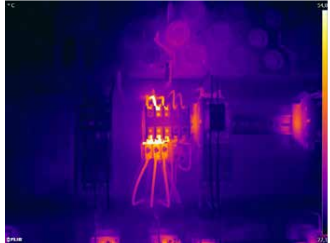
The middle phase of this motor protection switch looks abnormal. This could indicate increased resistance at the terminal connection.
