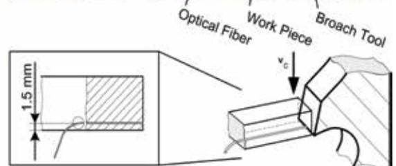
*The experimental set-up combines the FLIR SC7600 (infrared camera) with the optical fiber of the 2-colour pyrometer. In the example, the tool is moving down. As part of the experiment, a chip of just a few micrometers is removed from the tiny work piece at very high speed.*
