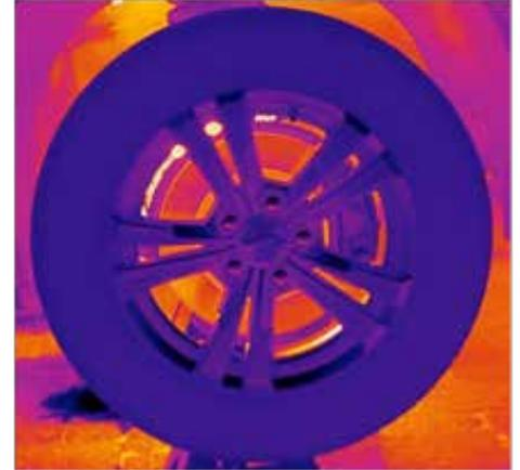
Cooled thermal Camera Image of Rotating Tire
