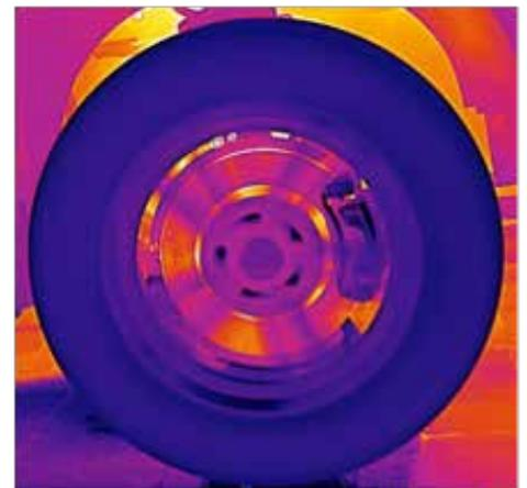
Uncooled Thermal Camera Image of Rotating Tire
