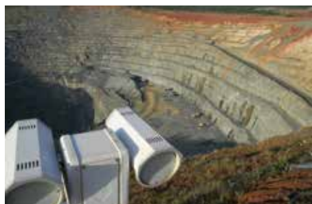
The FLIR PT-602CZ thermal imaging pan/tilt camera that is able to detect motion within a 6 km radius from nominal ground level.
