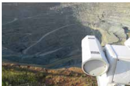
The FLIR PT-602CZ thermal imaging pan/tilt camera that is able to detect motion within a 6 km radius from nominal ground level.
