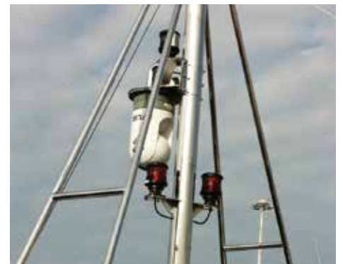
The FLIR M-324XP has been mounted in the "ball down" position on board of the pilot boat.
