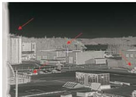
DDE applied - all targets can be observed simultaneously
