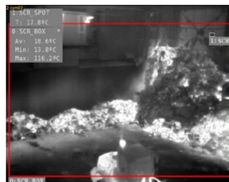
*The FC-Series R cameras measure the actual temperature of the waste piles and, whenever a predefined temperature threshold is reached, they issue an alarm.*
