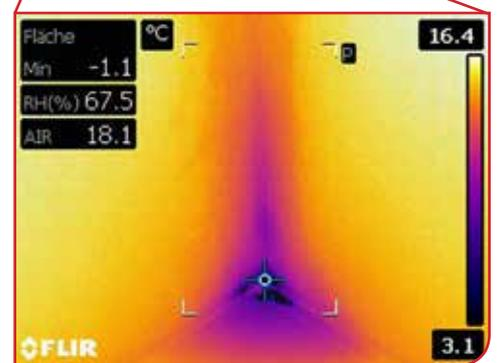
Frank Lochow, an employee of Meyer Malereibetrieb GmbH, examines a spot affected by moisture using the FLIR E50bx thermal imaging camera and the FLIR MR77 moisture meter.
