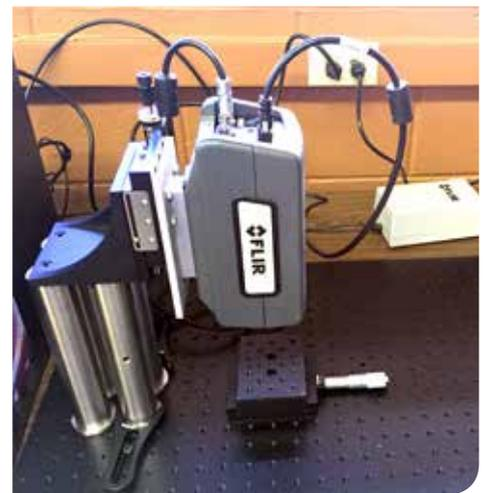
*In a typical test experiment, microheater lines on a substrate are connected to a power source. The device is heated up through Joule heating. Thus, the temperature field of the substrate evolves as a function of time.*
