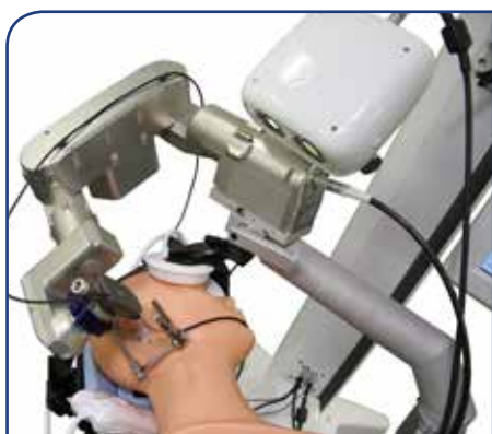
Researchers from the University of Bern have been working on a surgical robot which is able to only drill a small hole in the skull behind the ear through which the cochlear implant can be inserted.
