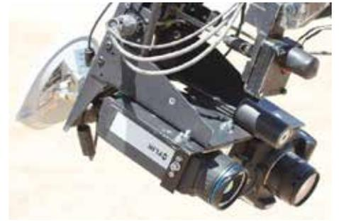
Next to a FLIR A655sc camera, the USDA team also makes use of an RGB camera, an IR thermometer, a multi-spectral camera and a GPS. All this equipment is attached to a boom that has been mounted on the tractor.
