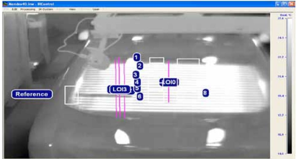
*The special software tool that Rato supplied Ford Genk with compares the temperature measurements the FLIR A320 thermal imaging camera made along the purple lines.*
