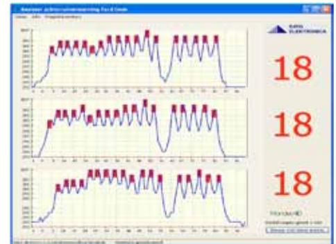
*The temperature readings result in a graph that should have exactly as many peaks as the car’s rear window has heating elements. If one of these peaks is missing on the graph that indicates a defective heating element.*
